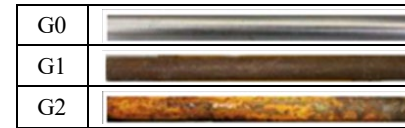
Fig. 2. Rebar inside specimen
