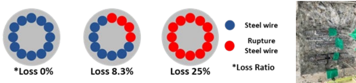
Fig. 2. Schematic of the artificial rupture of the internal tendon
