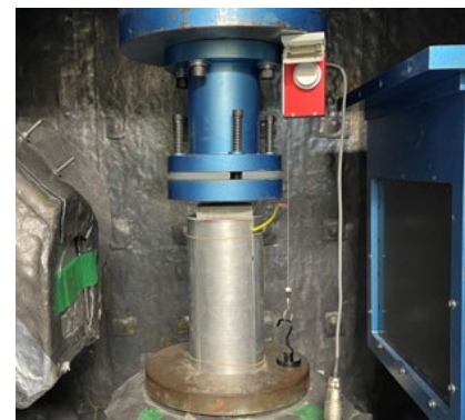
(c) X-ray tomography with loading
