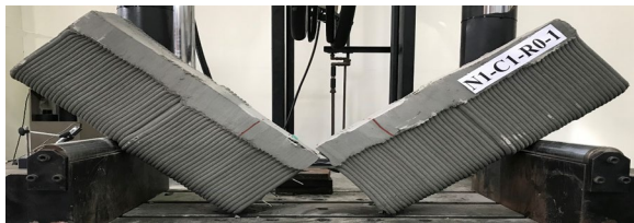
Fig. 3. Failure pattern of 3D printed beam without rebar and filling concrete
