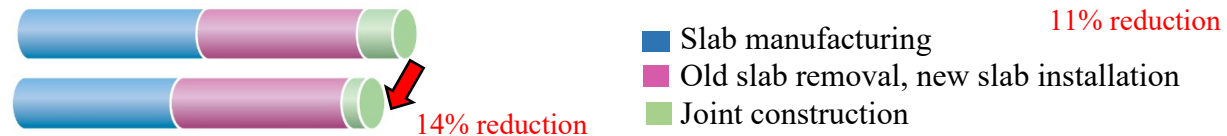
Fig. 4. Productivity (man-hours) comparison of loop joints and ELSS joint
